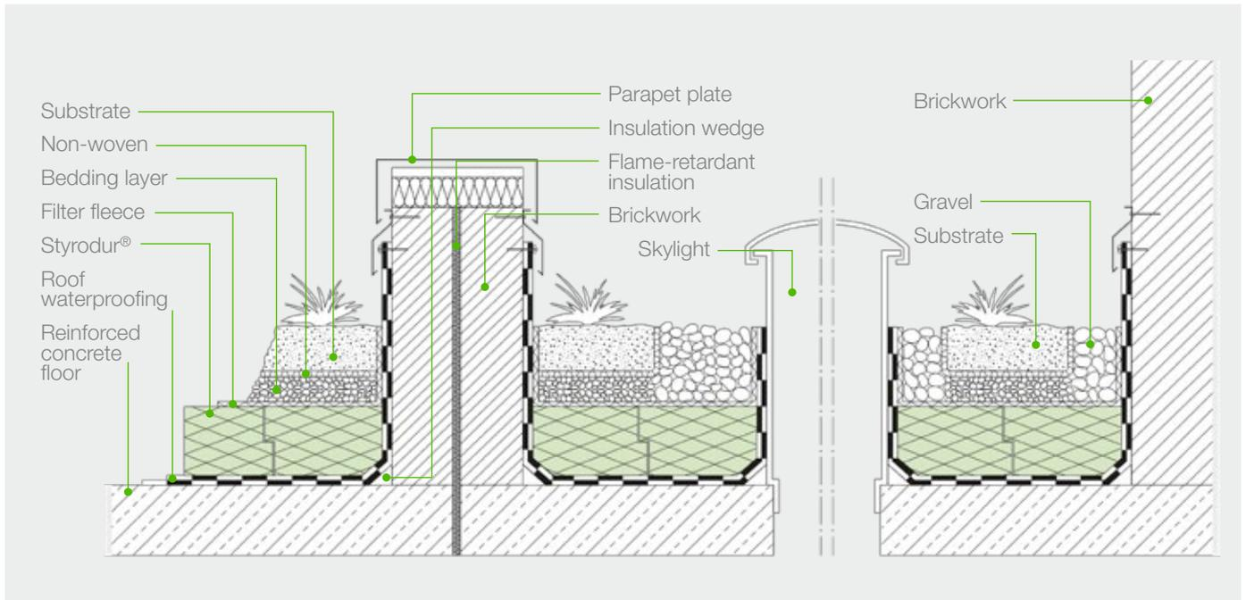
Fig. 36: Fire section of a flat roof with extensive greening.
