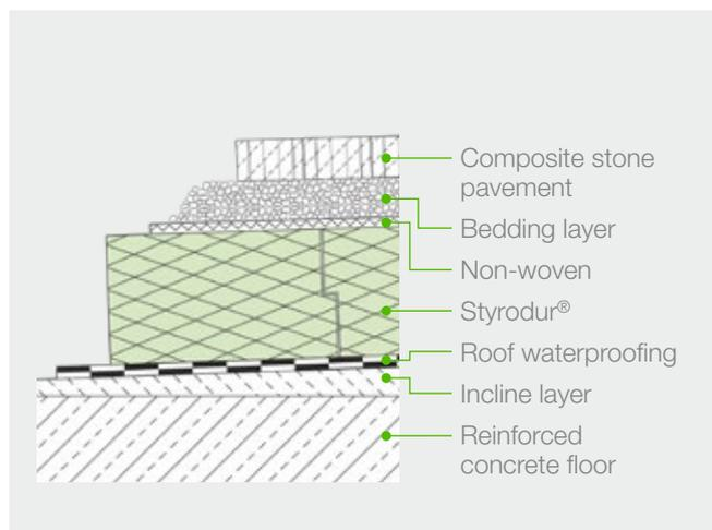
**Fig. 44:** Parking roof design with composite stone pavement on a bedding layer.
