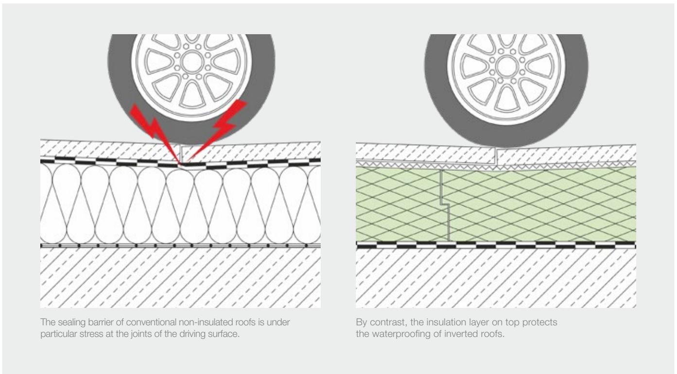
The sealing barrier of conventional non-insulated roofs is under particular stress at the joints of the driving surface.
