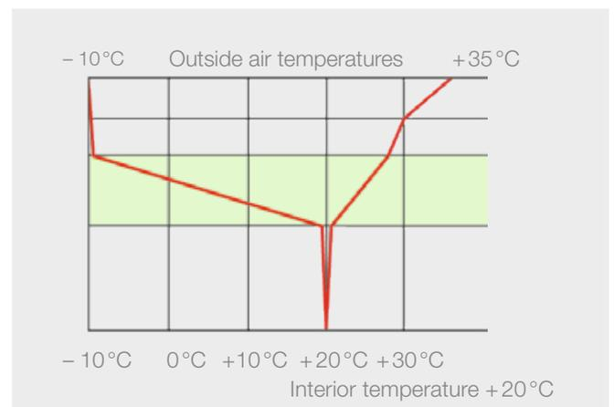
Fig. 21: Temperature profile of an inverted green roof.
