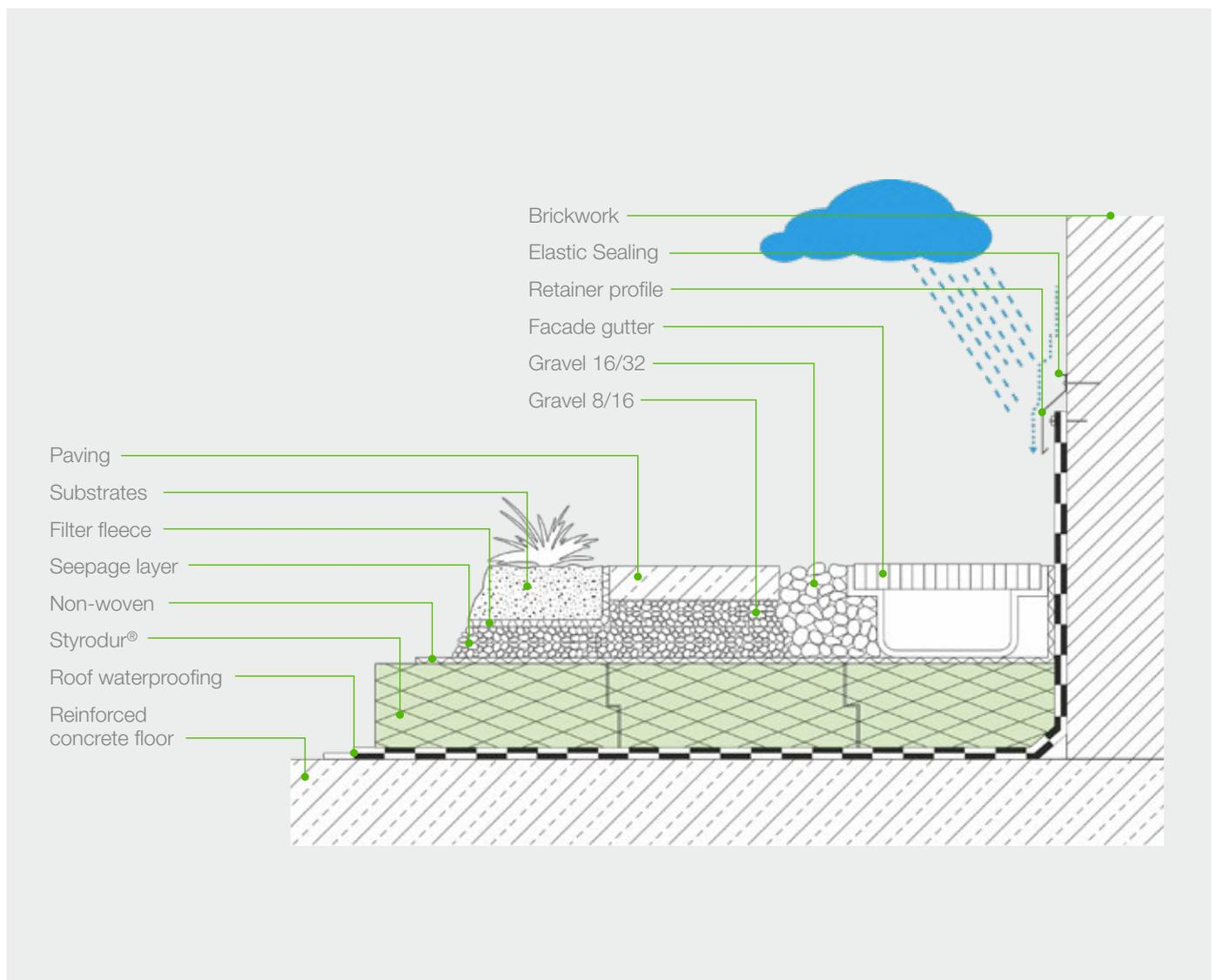
**Fig. 34:** Inverted green roof connection to a rising wall with facade gutter.
