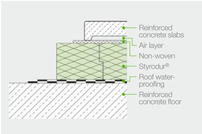
**Fig. 41:** Parking roof with large-size reinforced concrete slabs on pavement slab supports.
