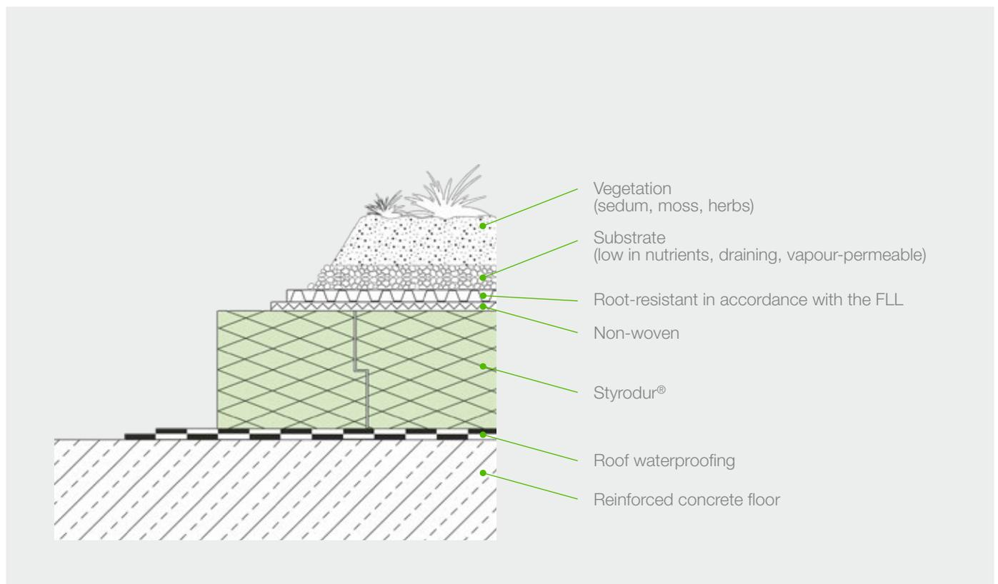
Fig. 26: Profile of an extensive green inverted roof.
