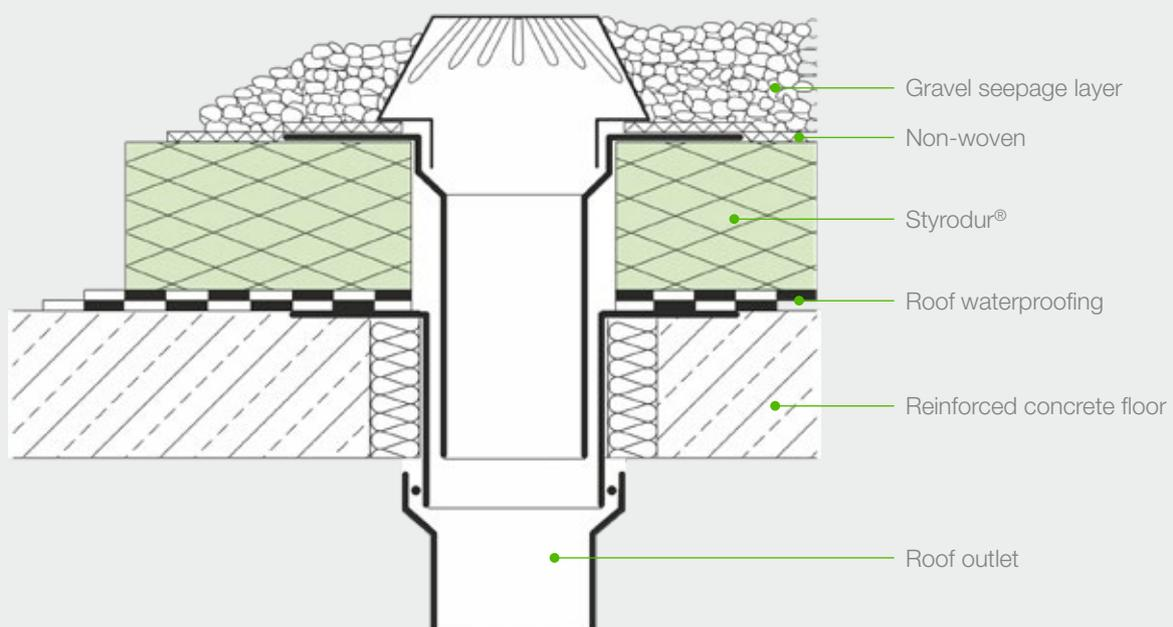
Fig. 8: Roof outlet with two drainage levels for draining the roof above and below the insulation layer.
