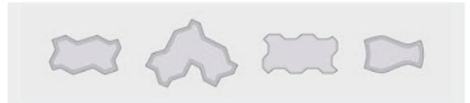
**Fig. 46:** Stone shapes for stable pavement.
