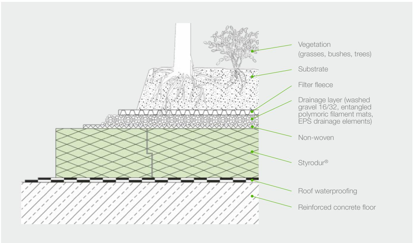
**Fig. 28:** Profile of an intensive green inverted roof.
