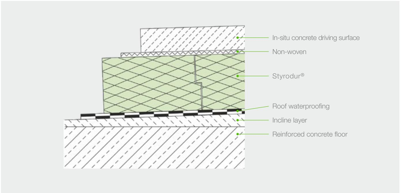
**Fig. 48:** Basic outline of a parking roof with in-situ concrete driving surface on an inverted roof construction with Styrodur®.
