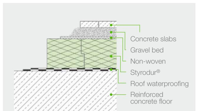
Fig. 38: Profile of an inverted patio roof with concrete slabs on a gravel bed.
