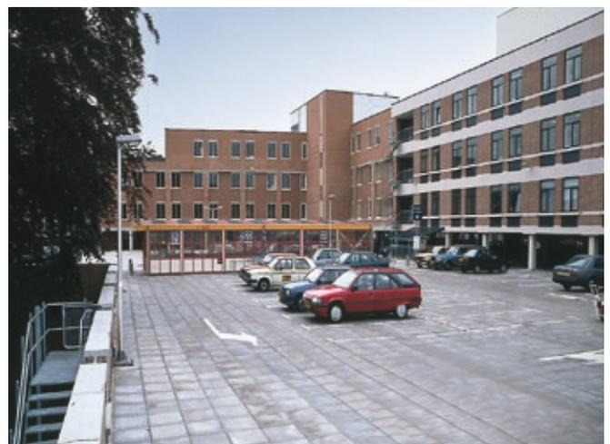
**Fig. 43:** Parking roof with concrete slabs laid on an inverted roof with Styrodur®.
