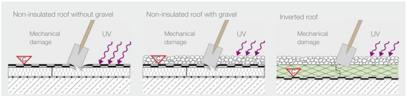
**Fig. 4:** An advantage of the inverted roof system is that the insulation material on top of the roof waterproofing protects it from high temperature fluctuations, thermal shocks, mechanical damage, and the sun's UV radiation.
