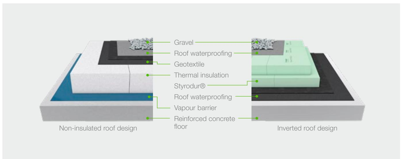
**Fig. 2:** Comparison of non-insulated and inverted roof designs.
